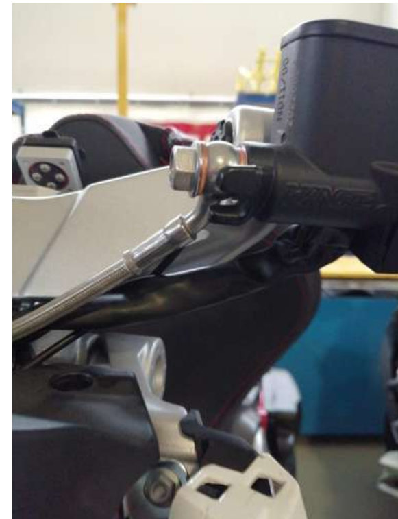
OEM BRAKE LINE FITMENT LE
