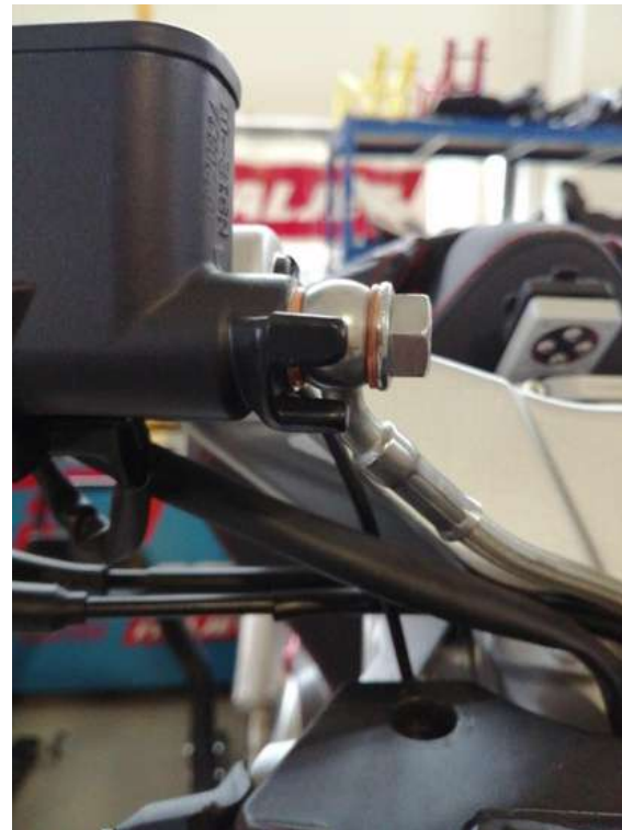
OEM BRAKE LINE FITMENT RH
